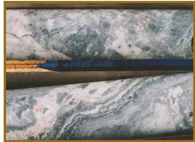
Multiple episodes of vein formation at the Tommy Vein (TS05-108) returned 12.6 g/t gold and 66.8 g/t silver across 3.9m
